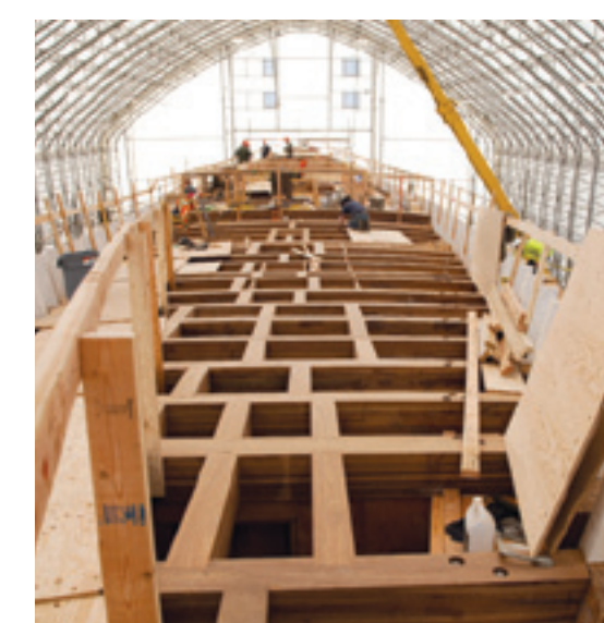
THIS PAGE: SOME PARTS OF THE BOAT WERE SAVED BUT THE HULL HAD TO BE RECONSTRUCTED. THE PRIMARY TIMBER IS ANGELIQUE, A DENSE HARDWOOD SIMILAR TO TEAK
