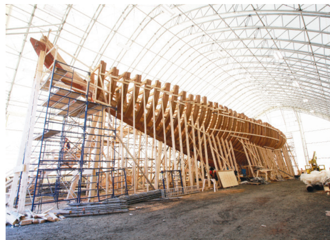
THIS PAGE: SOME PARTS OF THE BOAT WERE SAVED BUT THE HULL HAD TO BE RECONSTRUCTED. THE PRIMARY TIMBER IS ANGELIQUE, A DENSE HARDWOOD SIMILAR TO TEAK
