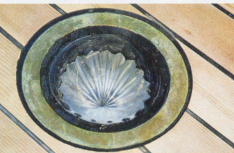
Bronze deadeyes on the shrouds (top, left) are strung with Spectra line. A modern block rides on a bronze traveler (top, right). Lignum vitae parrel beads (right) are tied to a carbon-fiber gaff with Spectra line. Classic deck prisms (above)—there are six altogether—light Maggie B's interior.
