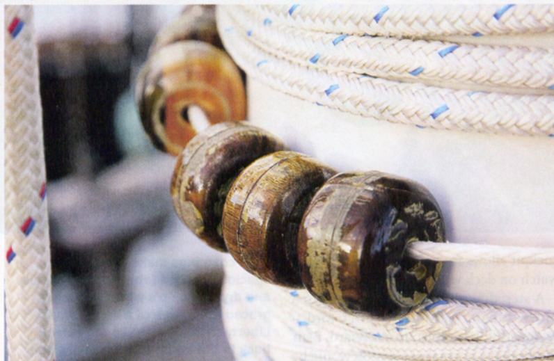
Bronze deadeyes on the shrouds (top, left) are strung with Spectra line. A modern block rides on a bronze traveler (top, right). Lignum vitae parrel beads (right) are tied to a carbon-fiber gaff with Spectra line. Classic deck prisms (above)—there are six altogether—light Maggie B's interior.
